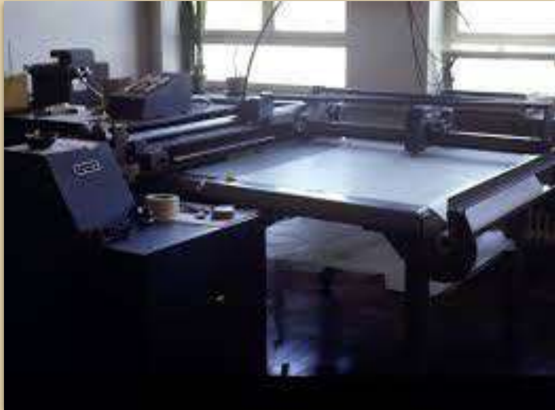
drawing machine ZUSE GRAPHOMAT Z64 1964 | 0.06 mm
