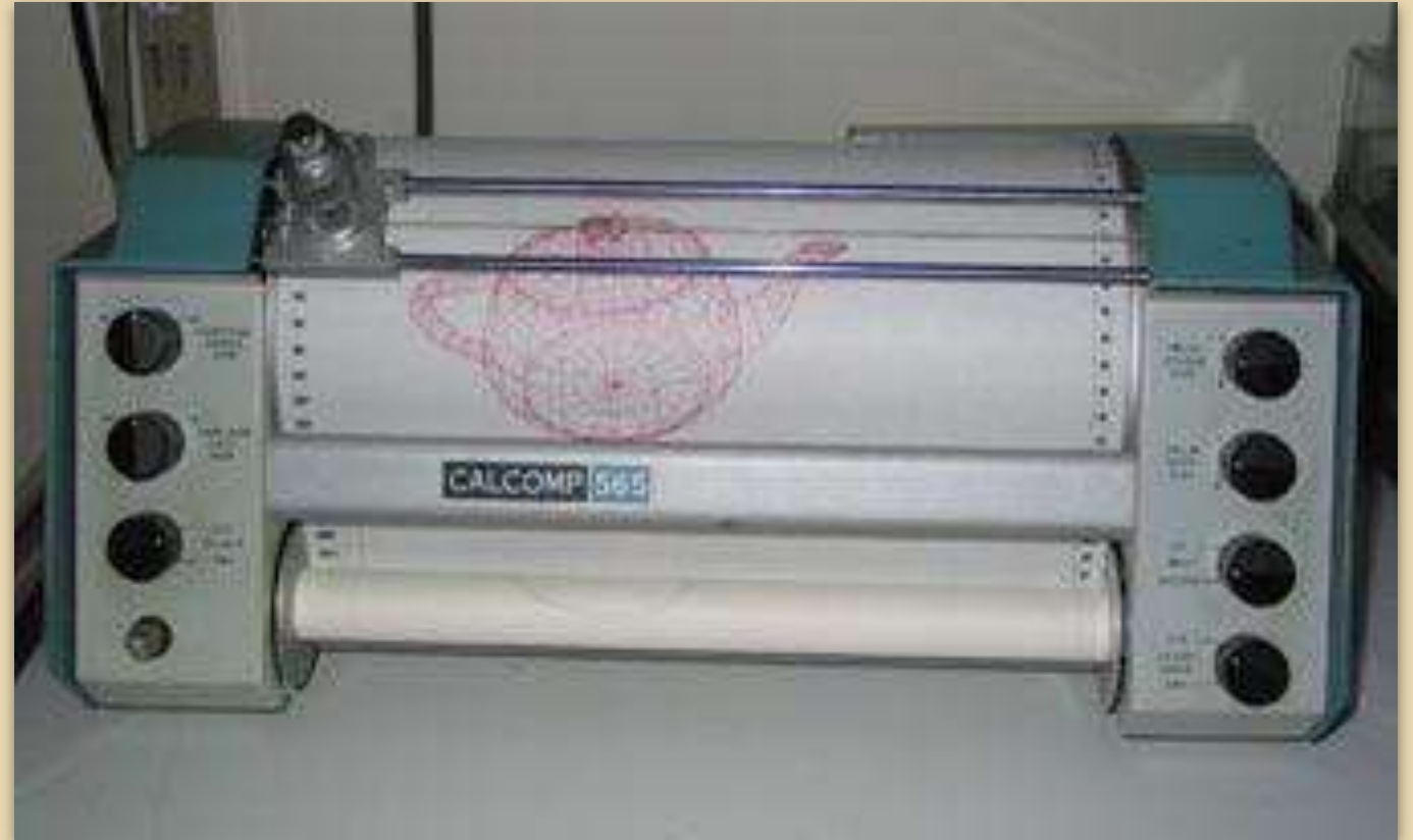
plotting machine Calcomp 565 1959 | 0.25 mm
